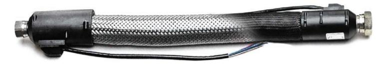
For the conveyance of liquids and gases under regulated temperatures - operating temperature range from 30°C to 260°C (86 to 500 °F), special versions up to 350°C (662 °F). Different diameters of internal hose combined with an extremely wide range of screw fittings and electrical connectors enable all technical and production process demands to be met.
