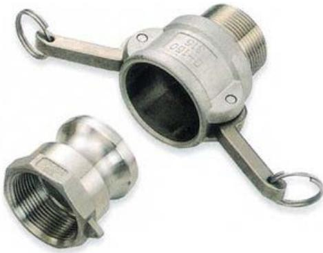
CAM-LOCK couplings were developed in order to obtain a quick and secure connection between two pipes. Simply insert the male connector into the female by placing the seal of the first one on the edge of the second and then lower the two eccentric levers to lock the fitting.
