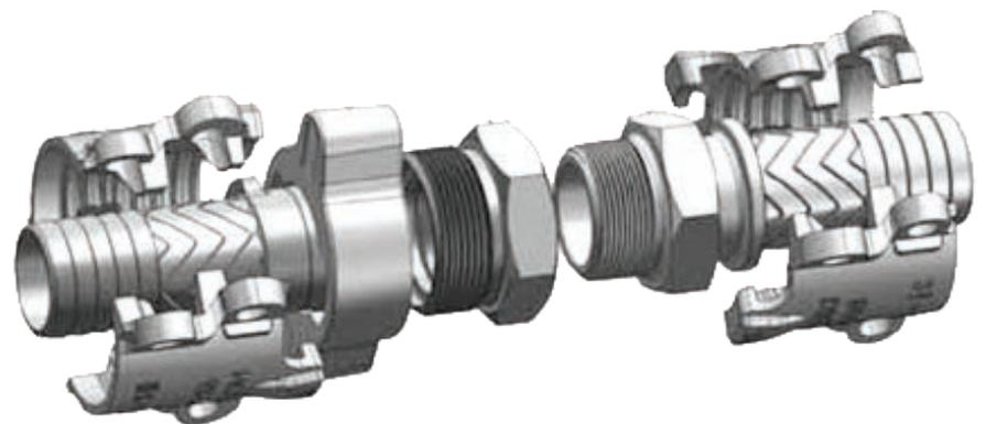
It consists of a special collared hose stems (Ground Joint), iron clamps (Interlocking Clamp) and spud. When properly installed, the gripping fingers on these clamps engage over the collar of the stem to prevent coupling blow-out.
