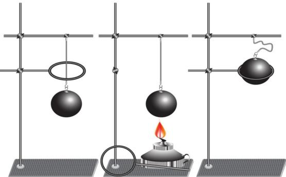
Heating metals to make them fit in other parts, taking advantage of the metal dilatation properties, has been a common practice for centuries.
