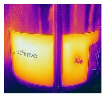
Bio reactor application with thermography checking. Heat is provided and transferred with perfect homogeneity, even on vast surfaces.
